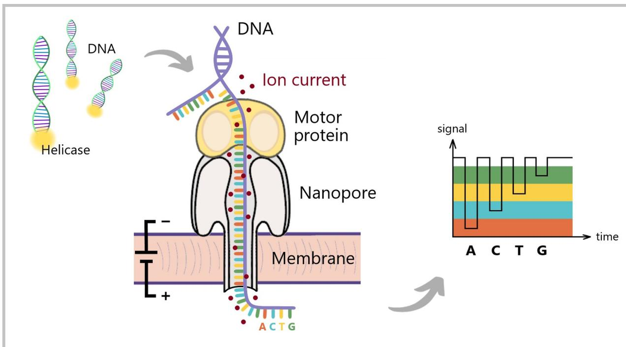
Fig. 45: Oxford Nanopore technology (schematic representation)
