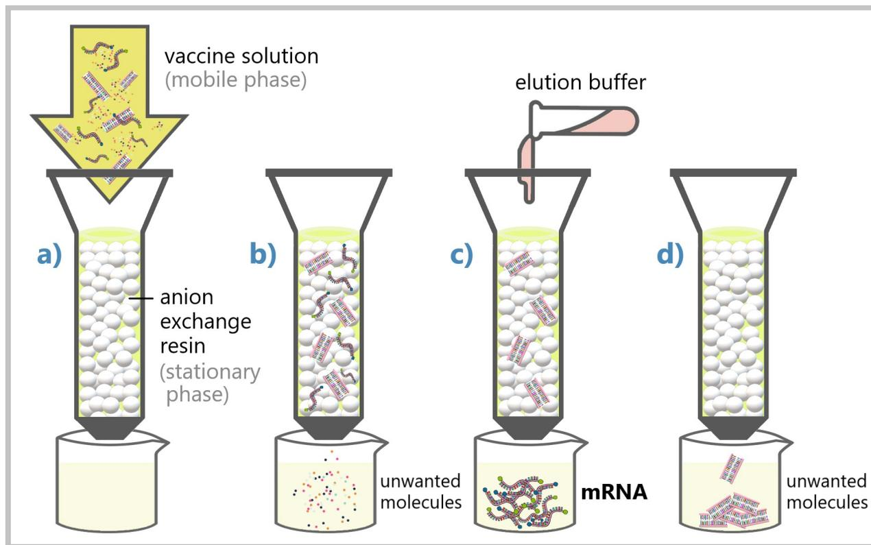
Fig. 38: Schematic representation of anion exchange chromatography
