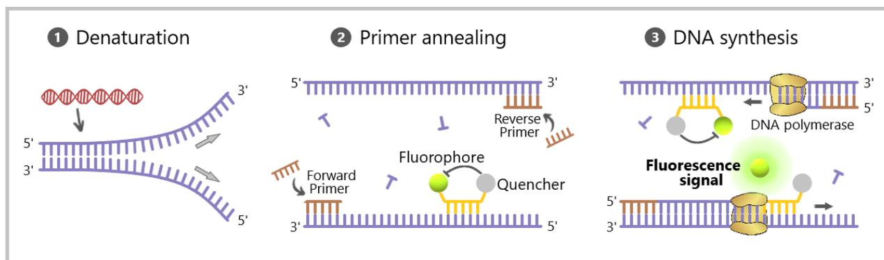
Fig. 41: Probe-based qPCR (schematic representation)
