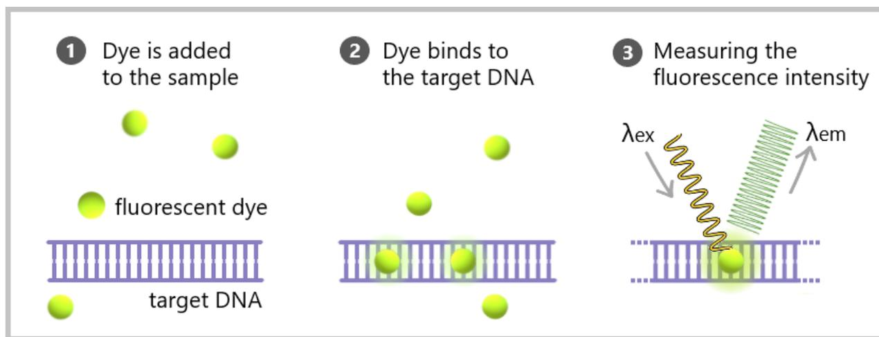
Fig. 42: Fluorometry with DNA Dyes (schematic representation)
