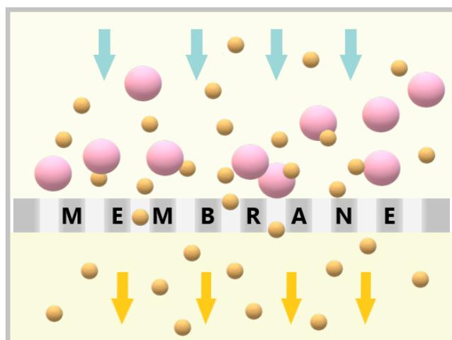
Fig. 32: Only smaller molecules pass through the membrane
