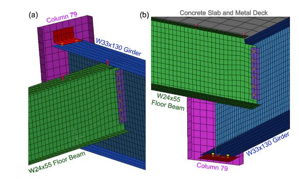
Figure 3.9 Figure 8-23 of the NIST report showing NIST's finite element analysis of the Column 79 and girder A2001 seated beam connection.
