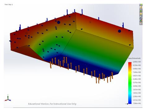
Figure 2.9 Temperature distribution of the unit floor slab.
