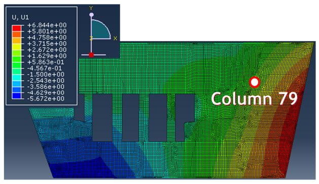
Figure 2.61 Movement in *x*-direction at Floor 13.
