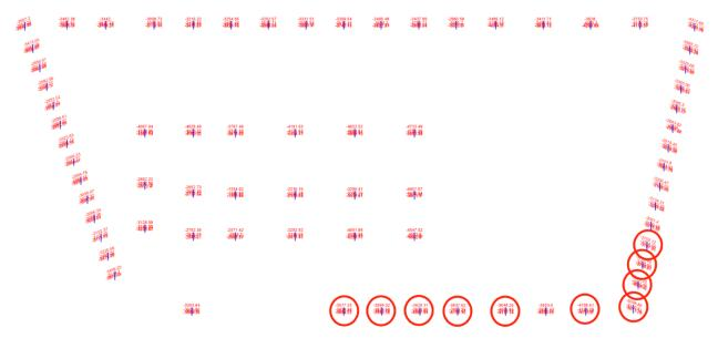
Figure 4.10: Linear static analysis results show that the failure of Columns 76 to 81 overloads 10 exterior columns (circled in red) around the southeast corner, but not the next row of core columns to the west (not circled in red).
