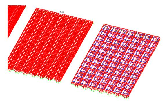
Figure 2.27 Models of floor slabs with different meshing.
