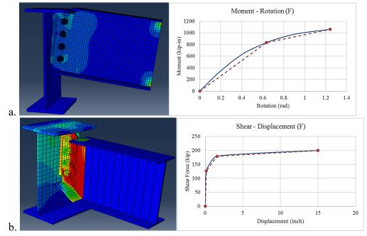
Figure 2.46 Fin connection (F): a. moment-rotation, b. shear-displacement.
