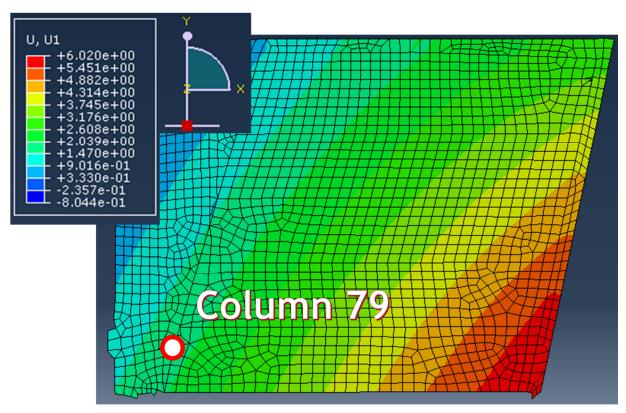
Figure 2.62 Movement in *x*-direction at Floor 13 around Column 79.
