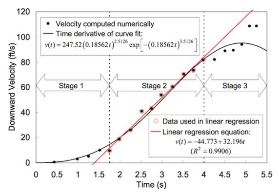
Figure 1.6 WTC 7 was in free fall for approximately 2.25 seconds over a distance of approximately 8 stories or 32.0 meters (NIST, 2008, NCSTAR 1A).
