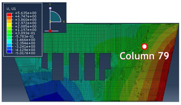
Figure 2.60 Movement in *x*-direction at Floor 12.
