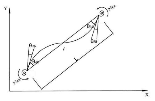
Figure 2.1 Rotational Nonlinear Springs
