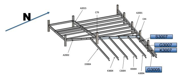
Figure 3.1 Member identification for the finite element analyses discussed below.
