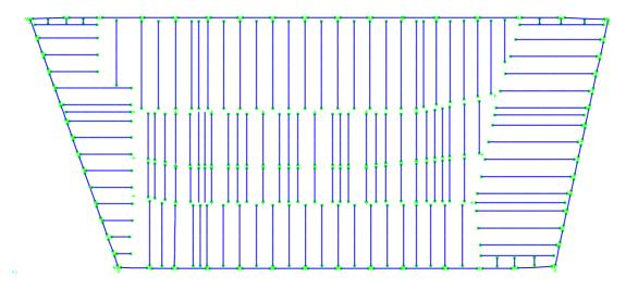
Figure 2.54 Beams on Floors 12 and 13 that had shear studs (NIST assumption).
