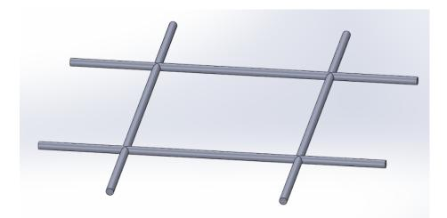
Figure 2.7 Welded wire fabric reinforcement.
