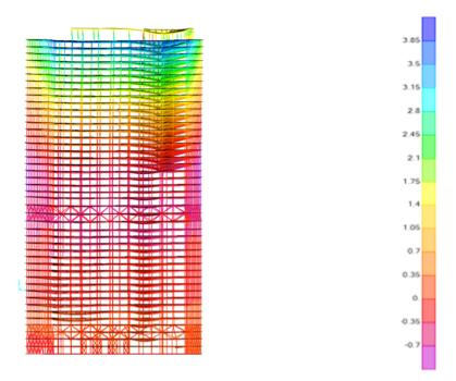
Figure 4.5: Columns 79, 80, and 81 are removed from Floor 29 to Floor 37. The building tilts to the east 3.85 inches. The penthouse does not collapse, thought its deflection increases.
