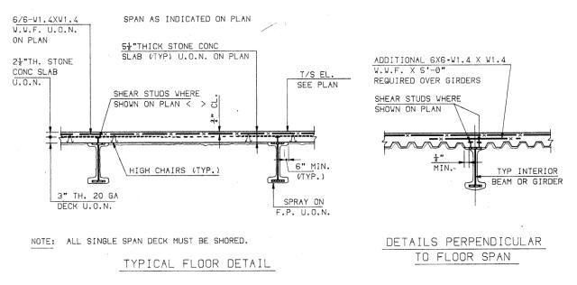
Figure 2.24 Typical floor detail of WTC 7.
