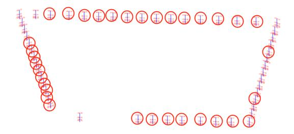
Figure 4.17: Linear static analysis results show that the simultaneous failure of all core columns leads to the failure of most exterior columns, causing the building to tip to the southwest. Only columns at the northwest corner and eastern side are not overloaded.
