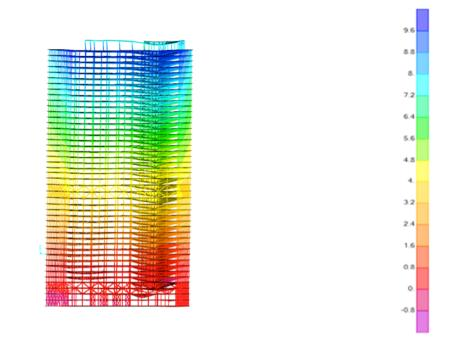
Figure 4.2: Columns 79, 80, and 81 are removed from Floor 6 to Floor 13. The building tilts to the east almost 10 inches. The penthouse does not collapse.
