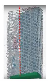
Figure 2.5 Progressive collapse separated into two parts.
