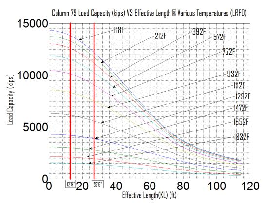
Figure 2.17 Load capacity of Column 79 versus effective length at different temperatures.
