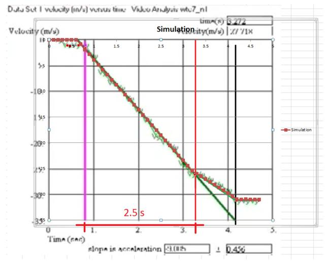
Figure 4.23: Velocity comparison between Chandler measurement (green plotted line) and UAF simulation (red plotted line). Bold green trend line illustrates free fall.
