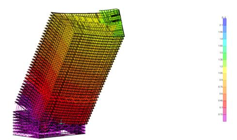
Figure 4.15: Visualization of linear static analysis, from the southwest, showing the building tipping to the southeast after the hypothetical failure of Columns 76 to 81.
