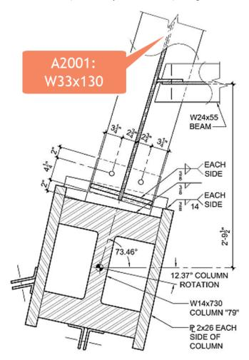
Figure 3.5 Plan View for Floor 13 at Column 79 and girder A2001 seat connection (Data from Frankel Steel Limited, 1985, Drawing 9114; figure prepared by Brookman, 2012).
