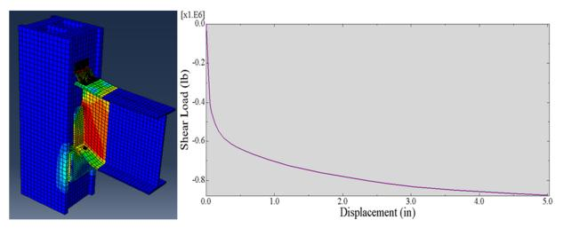
Figure 2.38 a. Connections modeling and shear-displacement nonlinear curve
