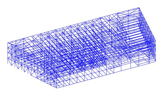
Figure 2.18 SAP2000 model for Floor 3 to Floor 7 with bracing.
