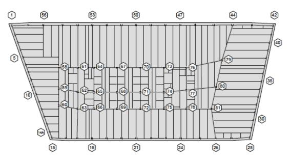
Figure 2.23 Column number layout of Floor 13 (NIST, 2008, NCSTAR 1A).
