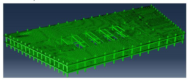
Figure 2.30 Floor 12 and 13 ABAQUS model.
