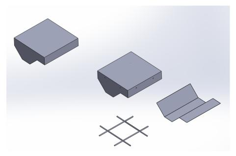
Figure 2.10 Equivalent floor slab and unassembled reinforced concrete slab of WTC 7.
