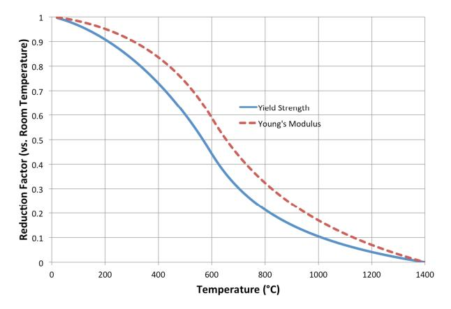
Figure 2.16 Mechanical properties of steel against temperature.
