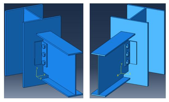
Figure 2.41 Knife connection sample ABAQUS model
