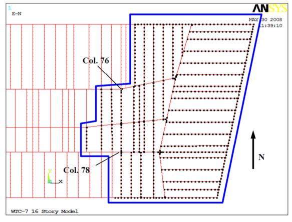
Figure 2.4 Area of floor where connection failure was modeled by NIST
