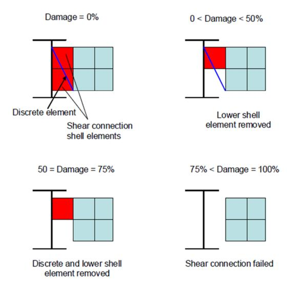
Figure 2.3 Shear connection damage; LS-DYNA model (NIST, 2008, NCSTAR 1-9, Vol. 2).
