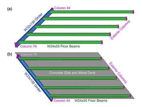
Figure 3.12 Figure 8-22 in the NIST report shows analysis results for G3005 with no lateral bracing condition (NIST, 2008, NCSTAR 1-9, Vol. 1, Page 350).
