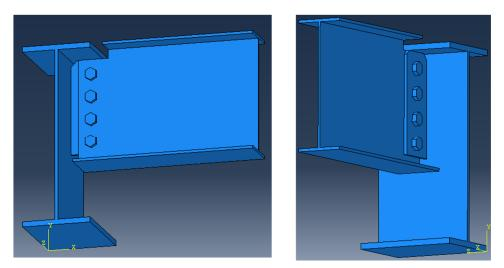
Figure 2.39 Fin connection sample ABAQUS model.
