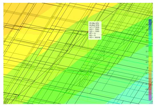
Figure 2.58 Displacement (inches) of the floor system surrounding Column 79.
