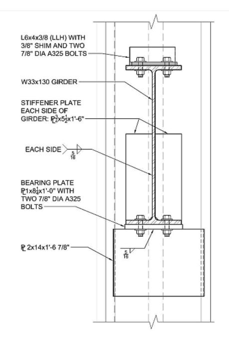
Figure 3.10 Section view at Floor 13 of Column 79 and girder A2001 seated beam connection, which shows stiffener plates on girder A2001 (Data from Frankel Steel Limited, 1985, Drawing 9114; figure prepared by Brookman, 2012).
