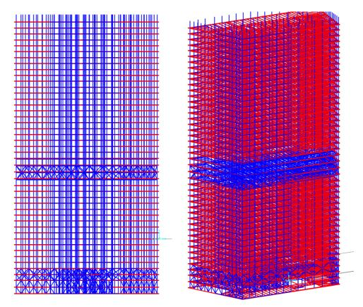
Figure 2.20 SAP2000 model of entire WTC 7 without roof.
