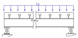
Figure 2.32 Simple beam and deck.
