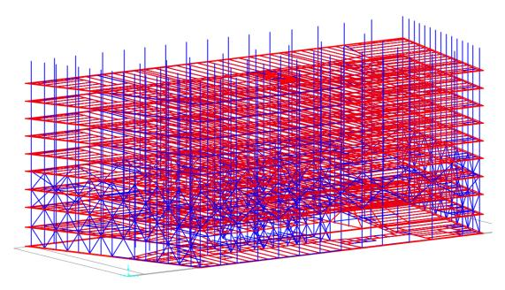
Figure 2.22 SAP2000 model for Floor 3 to Floor 12.
