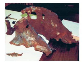
Figure 1.8 Steel from WTC 7 that experienced oxidation and sulfidation (FEMA, 2002).
