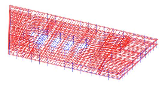
Figure 2.55 Assembly of Floors 12 and 13 in SAP2000.
