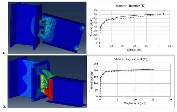
Figure 2.48 Knife connection (K): a. moment-rotation, b. shear-displacement.
