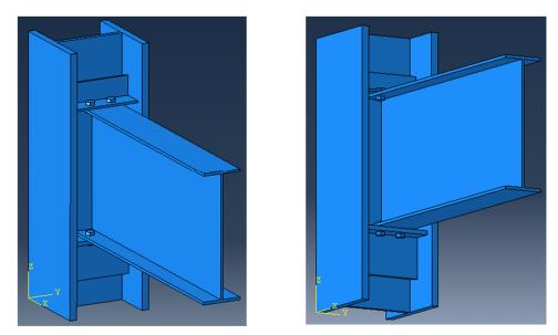
Figure 2.42 Seated top plate connection sample ABAQUS model.
