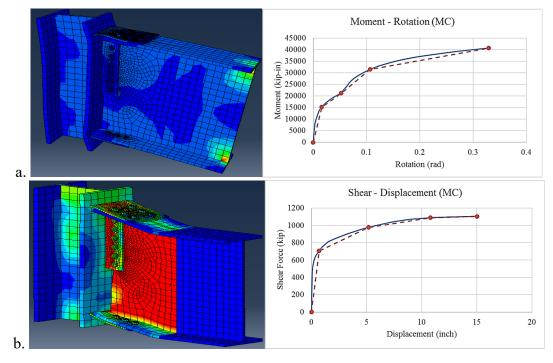
Figure 2.52 Moment connection (MC): a. moment-rotation, b. shear-displacement.
