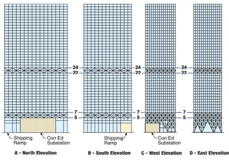
NOTE: Belt trusses located at floors 5-7 and 22-24.
