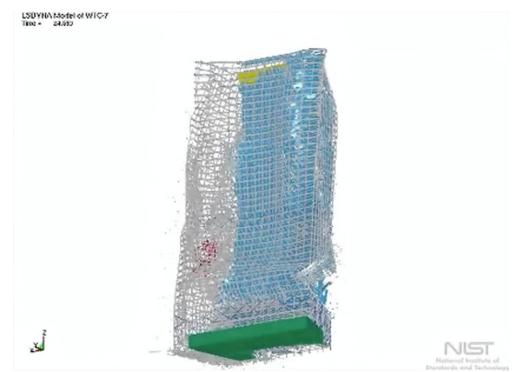
(b) NIST's progressive collapse simulation showing significant differential movements in the exterior (NIST NCSTAR 1A).
