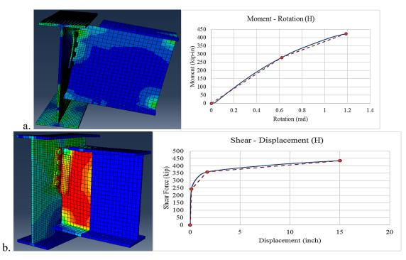
Figure 2.47 Header connection (H): a. moment-rotation, b. shear-displacement.
