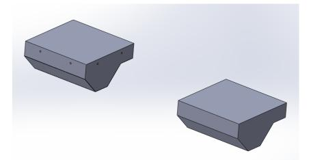
Figure 2.11 Equivalent floor slab and assembled reinforced concrete slab of WTC 7.
