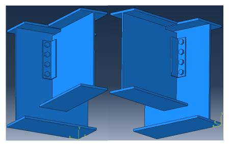
Figure 2.40 Header connection sample ABAQUS model.
