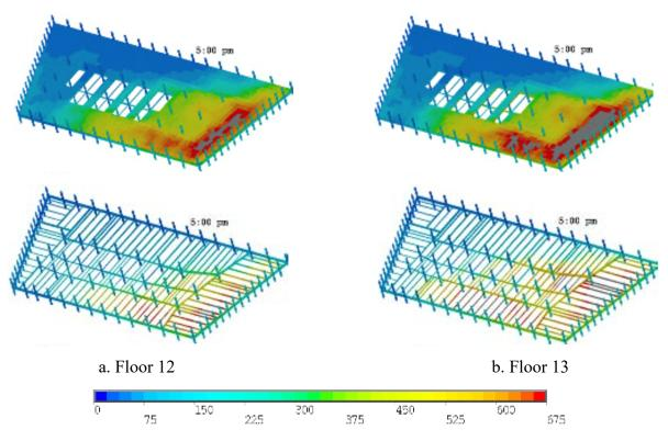
Figure 2.53 a. Floor 12, b. Floor 13 (NIST, 2008, NCSTAR 1-9, Vol. 2, Figures 10-36 to 10-39). The images at top represent the temperature distribution in the top layer of the concrete slab. The images at bottom represent the temperature distribution on the floor beams.
