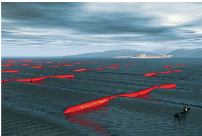
Figure 7.19: The Pelamis wave energy transformer floats on the ocean like a giant sea snake. It consists of several segments which move against each other and build up hydraulic pressure. This in turn drives a turbine. A new Pelamis generation is currently under construction.
